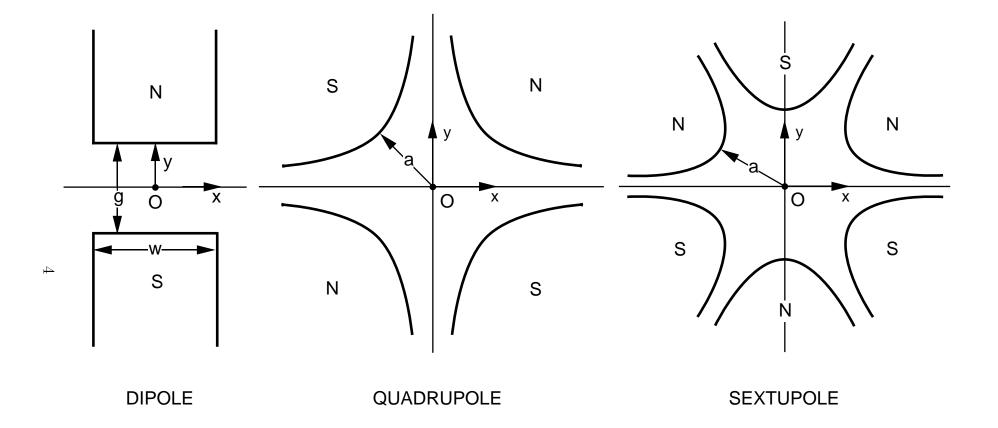
Illustration of the magnetic midplane (x axis) for dipole, quadrupole and sextupole elements. The magnet polarities indicate multipole elements that are positive with respect to each other. The coordinate system is right-handed, so that the beam particles will be emerging from the paper and moving into the face of the reader.
