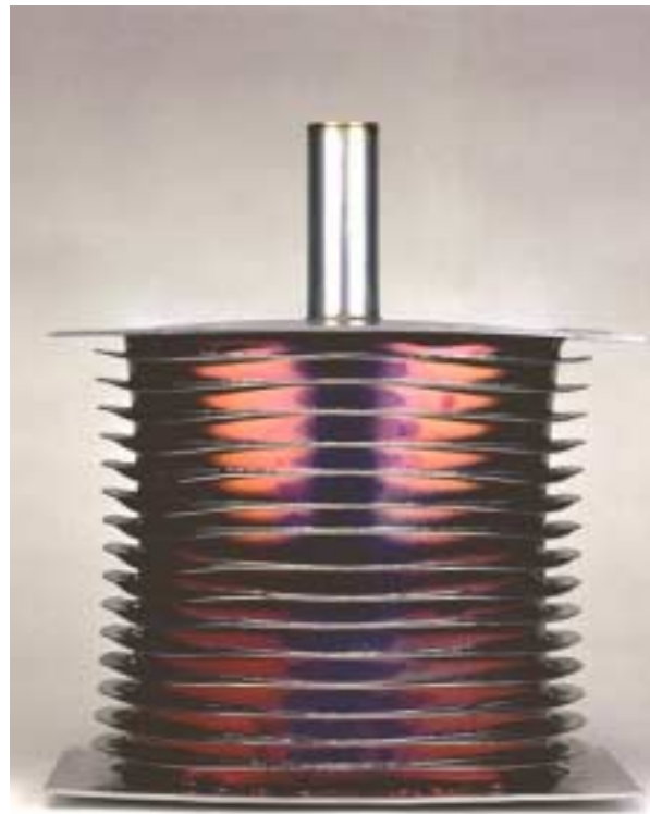
Figure 8.9. Photograph of Unsuccessful Prototype of Rib-Reinforced Vacuum Chamber
